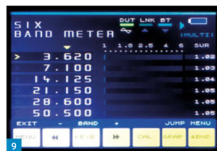
Fig. 9: SWR readings with active switch in circuit.
