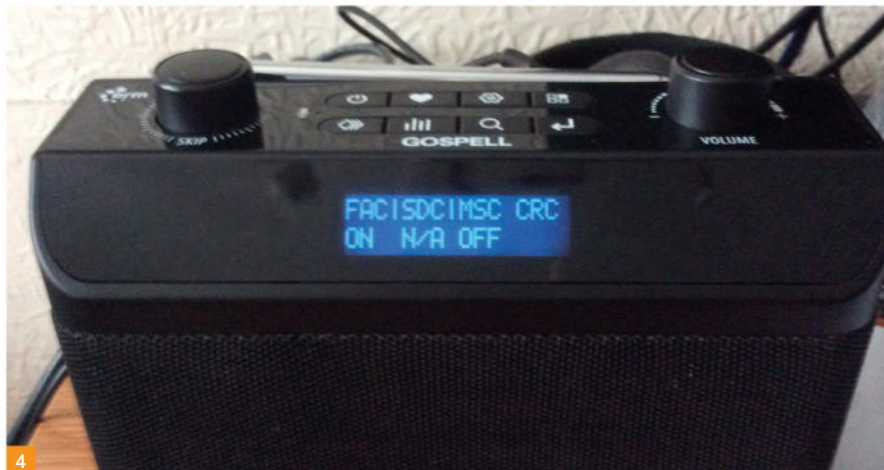
Fig. 4: All three status indicators must be ON to decode DRM audio. Fig. 5: The mode, bandwidth and encoding information. The FAC is always 4QAM.
