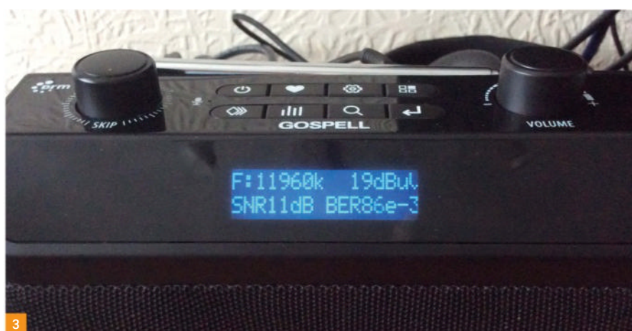
Fig. 1: Note the layout of the top panel and the wrap-around fabric cover on the body of the receiver. Fig. 2: The eight buttons on the top panel of the receiver. Fig. 3: Typically, the SNR needs to be about 12dB for an MSC using 16QAM and 17dB for 64QAM encoding.
