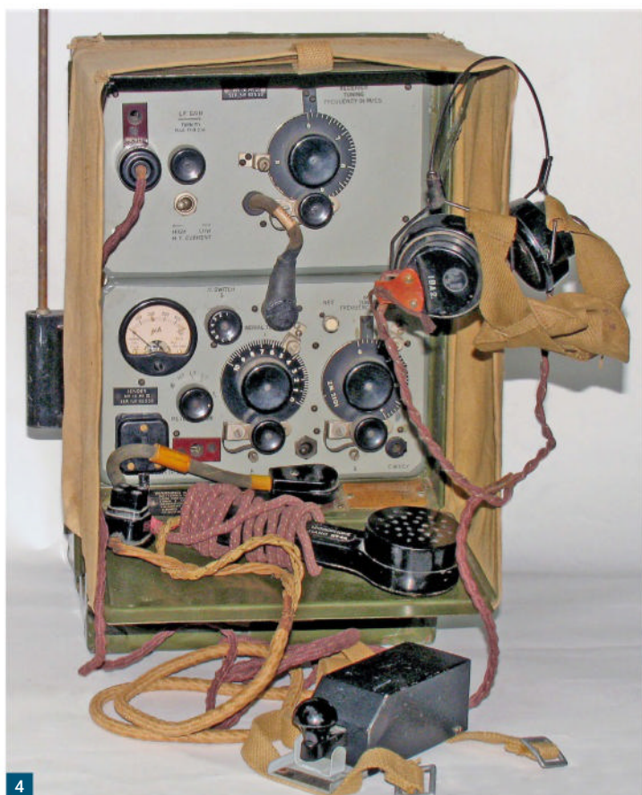
Fig. 1: Wireless Set No.11 (overleaf) was introduced in 1939 for use in tanks and AFVs, plus it was used by the Long Range Desert Group in the Western Desert from 1942 ( mapleleafup.net ). Fig. 2: Wireless Set No.19 is one of the most common WWII radios found for sale and continues to be popular with amateur radio enthusiasts. From 1941 it was the main set fitted to tank and AFVs ( image.wftw.nl ).
